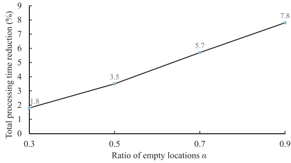
Fig. 5. The impact of storage location occupancy constraints on warehouse efficiency.
