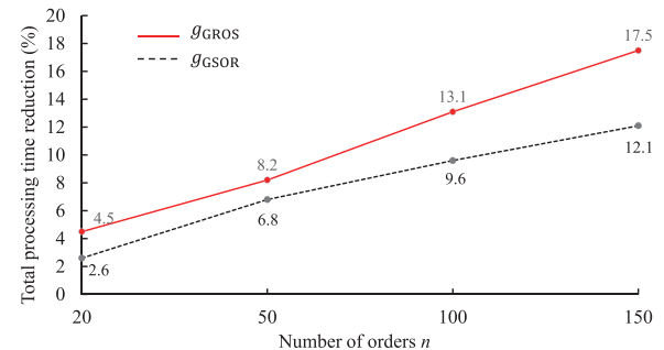
Fig. 3. Impact of the order quantity on the improvement of joint optimization.
