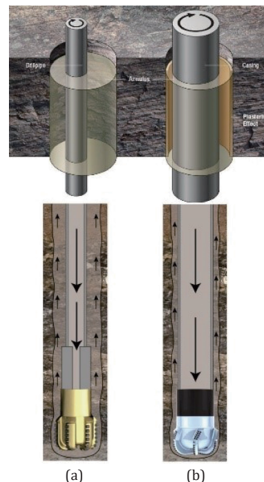
Fig. 9. (a) Conventional drilling, and (b) CwD wellbore geometry [22] .
