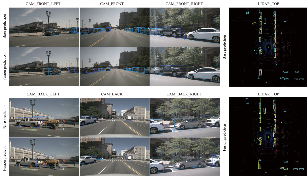
Fig. 4. Qualitative analysis of detection results. 3D bounding box predictions are projected onto images from six different views and BEV respectively. Boxes from different categories are marked with different colors and without ground truth. For BEV visualization, yellow means predicted boxes and blue ones are ground-truth, while LiDAR points are visualized as background.
