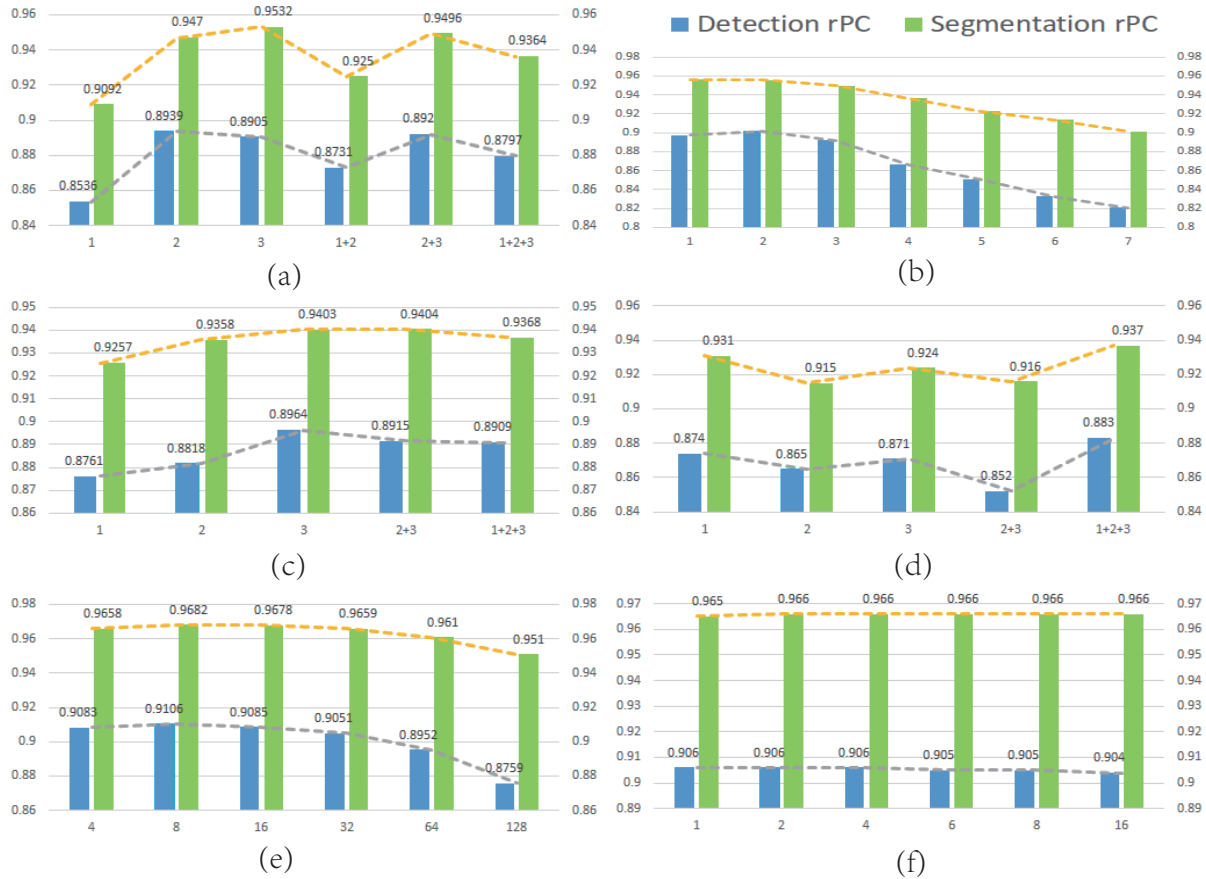
Fig. 5. Analysis experiments. (a) The effect of multi-scale features in PatchCore on robustness. “1”, “2”, and “3” represent the features from layer1, layer2, and layer3 in ResNet, respectively. (b) The effect of neighborhood size on the robustness of the domain aggregation module in PatchCore. (c) The effect of multi-scale features on robustness in Reverse Distillation. (d) Effect of multi-scale distillation in Reverse Distillation on robustness. (e) Effect of the number of FAM iterations. (f) Effect of the number of FAM reference features.
