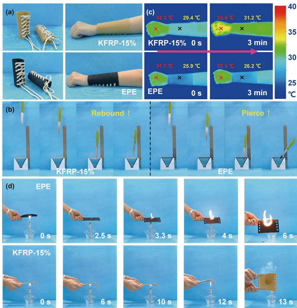
Fig. 7. (a) Photographs of the bracers based on KFRP-15% and EPE. (b) Infrared thermal images of bracers. (c) The process of the sharp knife impacting KFRP-15% and EPE in free fall. (d) Burning photos of the bracers based on KFRP-15% and EPE.
