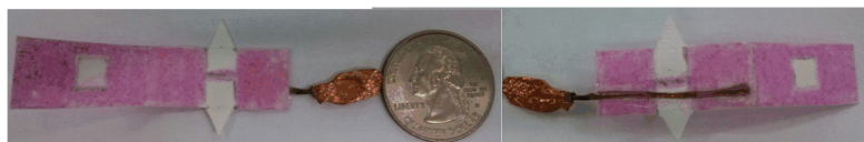
Fig. 2 The designed paper-based device
