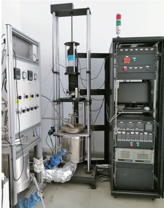
图 2 高温液态金属慢应变速率拉伸装置 Fig.2 Slow strain rate tensile test device with high temperature liquid metal
