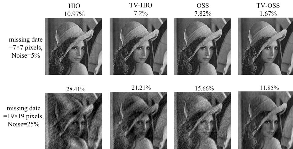
Fig. 6 Reconstruction results and reconstruction error coefficients of the four algorithms obtained under the best and worst simulation conditions
