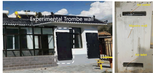
Figure 2. The experimental photos of the purified Trombe wall in Qinghai.
