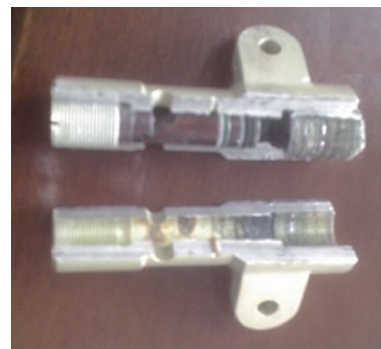
Fig. 12. Picture of IED transections after function test.
